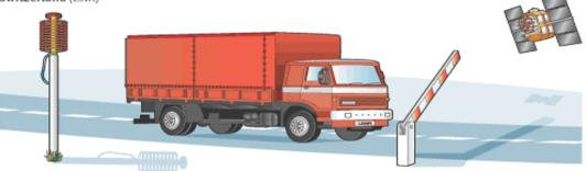
Microwave beacons activate and deactivate each truck's on-board unit (OBU) as it enters and leaves the country. The OBU determines distance travelled from the truck's tachograph. Satellite positioning (GPS) technology is used to verify the tachograph results. Both tachograph and GPS readings are stored on a smart card. The smart card is sent to the customs authority, which issues a bill.
