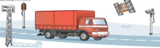
Readings from microwave beacons, GPS, the tacograph and an on-board gyroscope are combined by the OBU to determine the truck's position. The OBU calculates the toll and informs a central data-centre via the mobile-phone network, so a bill can be issued. Roadside cameras ensure that all trucks are registered with the system.
