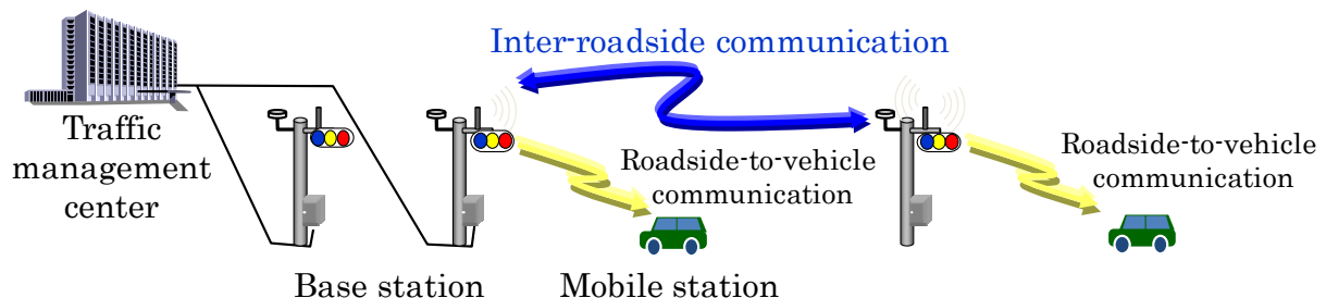
Figure R1.1 Example for roadside-to-vehicle communications and inter-roadside communications
