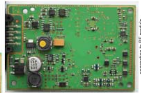
Back side (power supply)
